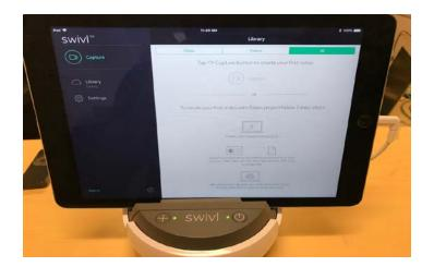
9. Once cables are plugged in and Swivl app is open, both lights on Swivl should be green as well as the lights on the marker.
