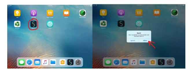
8. Once cables are plugged in, open Swivl app and when the notification pops up asking to allow the Swivl to connect, press 'Allow".
