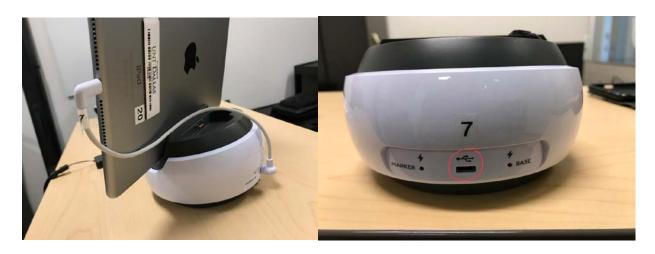
3. Plug the lighting port end of the cable to the charging port of the iPad and the mini USB end to the back of the Swivl.
