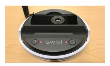
5. Light next to power button and + button will turn red when powered on (If they are both blinking this is an indication to charge the base).
