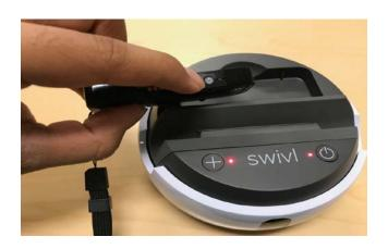
6. Remove marker from dock and hold down power button to turn on the maker.
