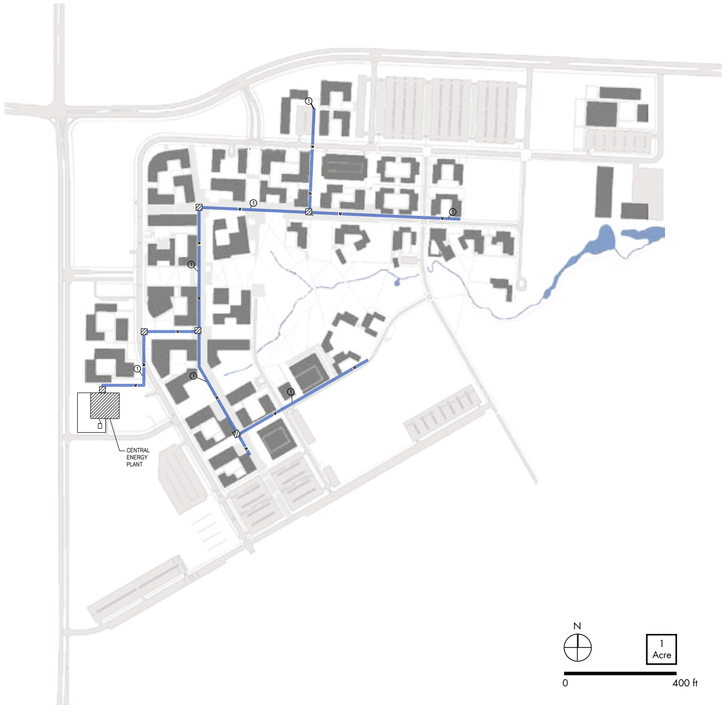
Figure 8.4 Chilled Water Loop
