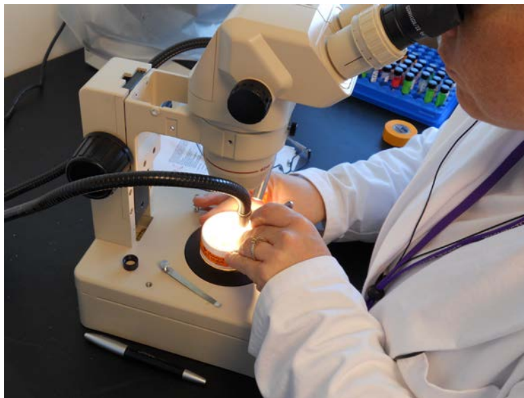
Figure 12. Microplastic fragments are extracted from the prepared sample during a microscope examination.
