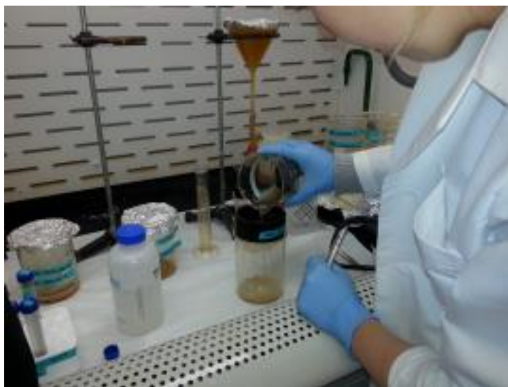
Figure 17. The lithium metatungstate solution is sieved and saved.
