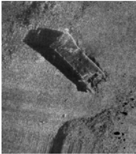
Figure 6. Side scan sonar image of a barge. There are many variables that affect the sonar data and how the resulting sonar records depict the seabed and various targets. Environmental conditions, such as wind, waves, currents, and density gradients from temperature or salinity changes, all influence the quality and interpretability of side scan sonar data.
