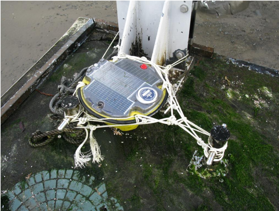
Figure 8: The tracking buoy is attached to the dock (Photo: WDFW)
