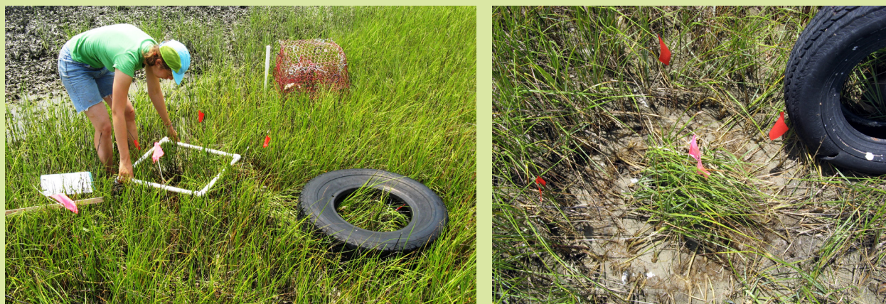
Figure 2. A researcher monitors a vehicle tire and blue crab trap that were experimentally deployed on a fringing salt marsh as part of an impact study in Beaufort, North Carolina (left). The impact footprint of a vehicle tire in a fringing salt marsh in Beaufort, North Carolina (right). Photo Credit: NOAA.
