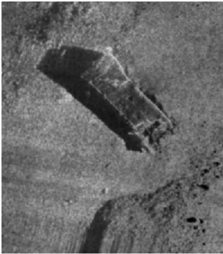
Figure 6. Side scan sonar image of a barge. There are many variables that affect the sonar data and how the resulting sonar records depict the seabed and various targets. Environmental conditions, such as wind, waves, currents, and density gradients from temperature or salinity changes, all influence the quality and interpretability of side scan sonar data.
