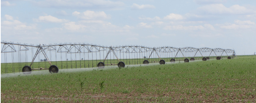
A straight pipe with water hoses spraying water rotate around a stationary spigot to irrigate crops.
