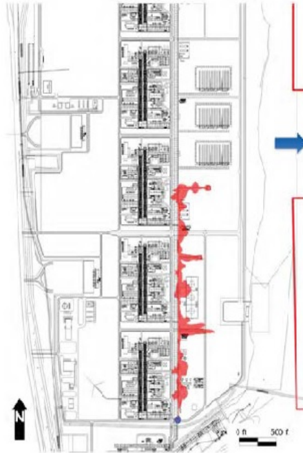
Figure 11: Time Composite Image of Vapor Dispersion for the Guillotine Release from the LNG Rundown Header at Liquefaction Train 1 (Scenario 5) with Wind from East.
