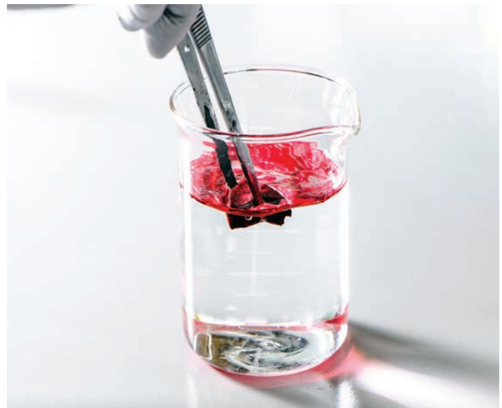
Cellulose nanofibril smart sponge absorbs oil that is floating on the top of the water. (Photo by Bryce Richter, University of Wisconsin)
