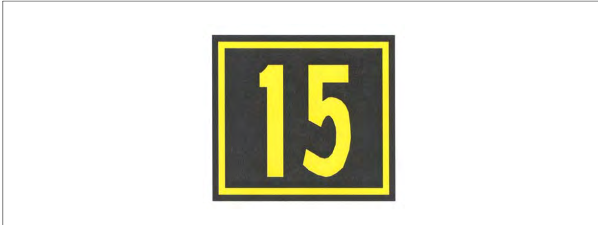
FIG AD 1.1-46 Runway Location Sign
