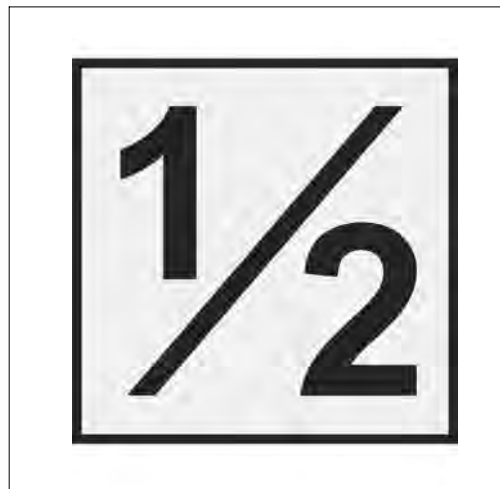
FIG ENR 5.7-1 Typical Runway Half-way Sign
