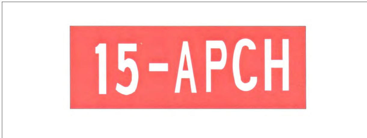
FIG AD 1.1-41 Holding Position Sign for a Runway Approach Area
