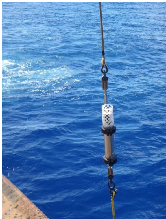
Hydrophone being lowered into the Challenger Deep trough in the Mariana Trench in 2015. (NOAA photo)
