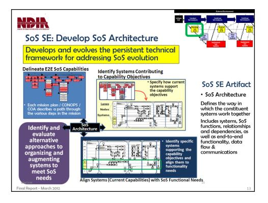
The next step is to develop the SoS Architecture, which includes systems, key SoS functions, relationships and dependencies, as well as end-to-end functionality, data flow and communications protocols. It is used to address possible changes in functionality, performance or interfaces. The architecture defines how constituent systems work together and may lead to with changes needed in system interfaces and functionality when key to cross-cutting SoS issues
