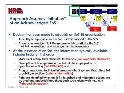
This approach assumes that the 'Initiate SoS step' in the wave model has taken place. This means that there is an organization responsible for the SoS and there is SoS SE support. However, as is the case with acknowledged SoS, the systems which support the SoS objectives maintain management and operational independence, and typically continue to support their original users.
