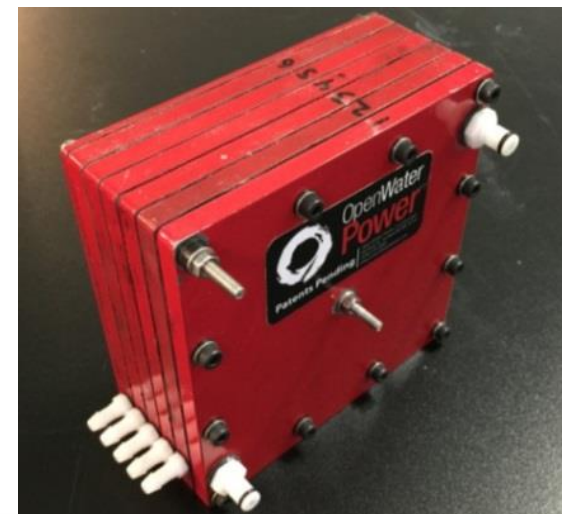
Aluminum-Seawater Fuel Cell
