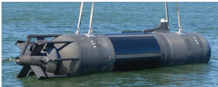
FIGURE D.4 Long-endurance unmanned undersea vehicle (UUV). SOURCE: Courtesy of the Applied Research Laboratory at Pennsylvania State University.
