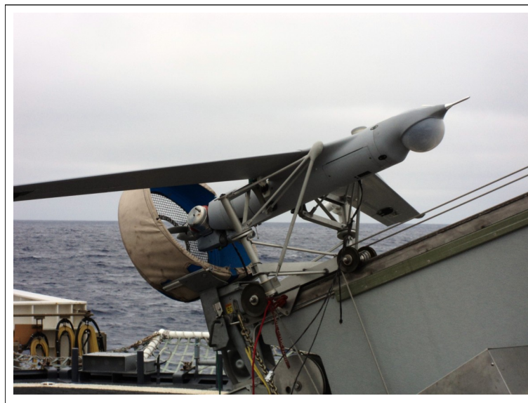
ConocoPhillips is working with Insitu for their ScanEagle operations. ScanEagle is launched via catapult (shown above) and recovered with a Skyhook. USCG photo by Cmdr. Jeff Vajda.
