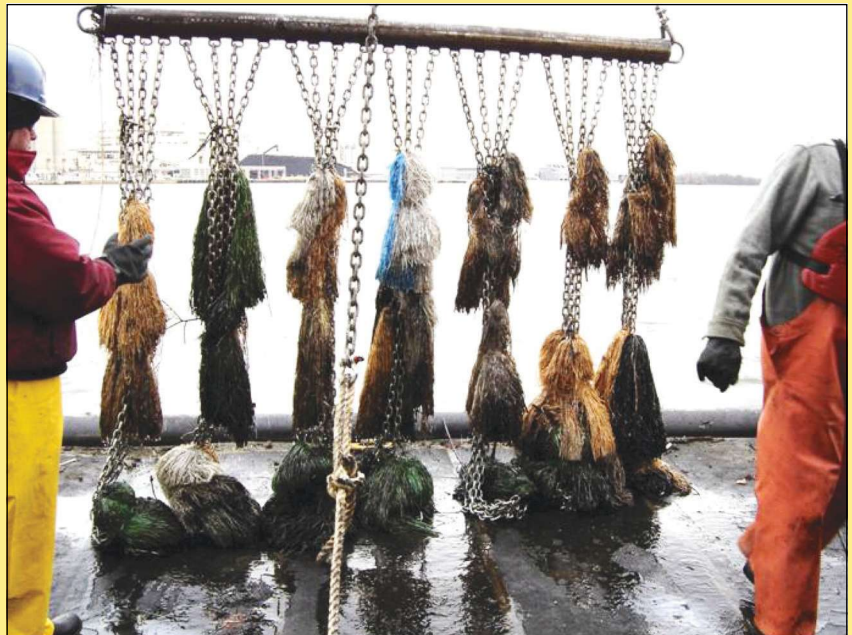
Sorbent material submerged oil recovery in the field. U.S. Coast Guard photo.
