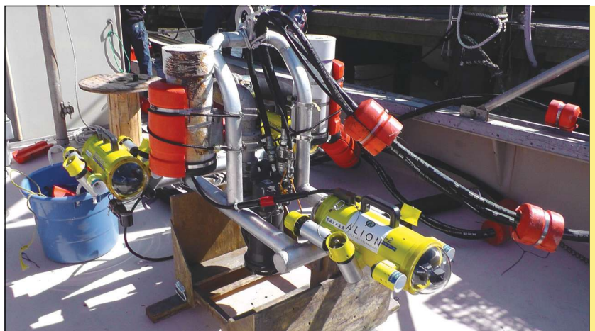
Updated system uses three ROVs. Photo courtesy of Alion Science and Technology.
