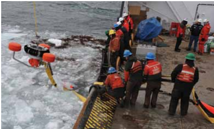
STRAITS OF MACKINAC - Crewmembers aboard the Coast Guard Cutter Hollyhock, homeported in Port Huron, Mich., use an oil-skimming device to recover peat moss, acting as a substitute for spilled oil, near Mackinac Island, Jan. 24, 2012. The crew of the Hollyhock is participating in a project led by the Coast Guard's Research and Development Center, showcasing techniques for removing spilled oil from a frozen environment. U.S. Coast Guard photo by Petty Officer 1st Class Matthew Schofield.
