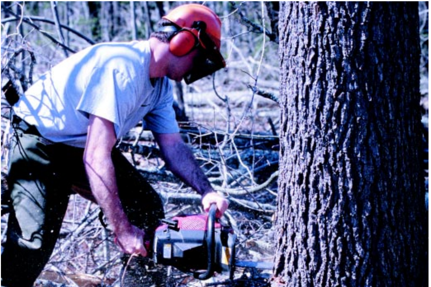
A logger wears a hardhat with logger face screen, hearing protectors, and chainsaw chaps. Photo by Eric Johnson
