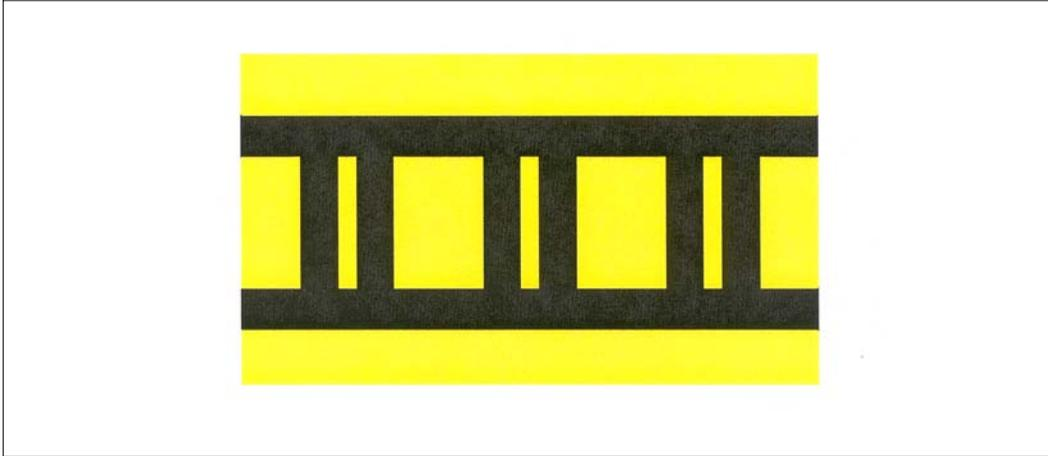
**4. ILS Critical Area Boundary Sign.** This sign has a yellow background with a black inscription with a graphic depicting the ILS pavement holding position marking as shown in FIG 2-3-34. This sign is located adjacent to the ILS holding position marking on the pavement and can be seen by pilots leaving the critical area. The sign is intended to provide pilots with another visual cue which they can use as a guide in deciding when they are “clear of the ILS critical area.”
