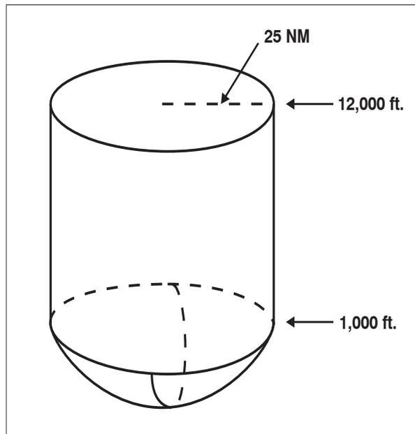
2. Within 25 NM, the bottom of the T service volume is defined by the curve in FIG 1-1-4. Within 40 NM, the bottoms of the L and H service volumes are defined by the curve in FIG 1-1-5. (See TBL 1-1-1.)
