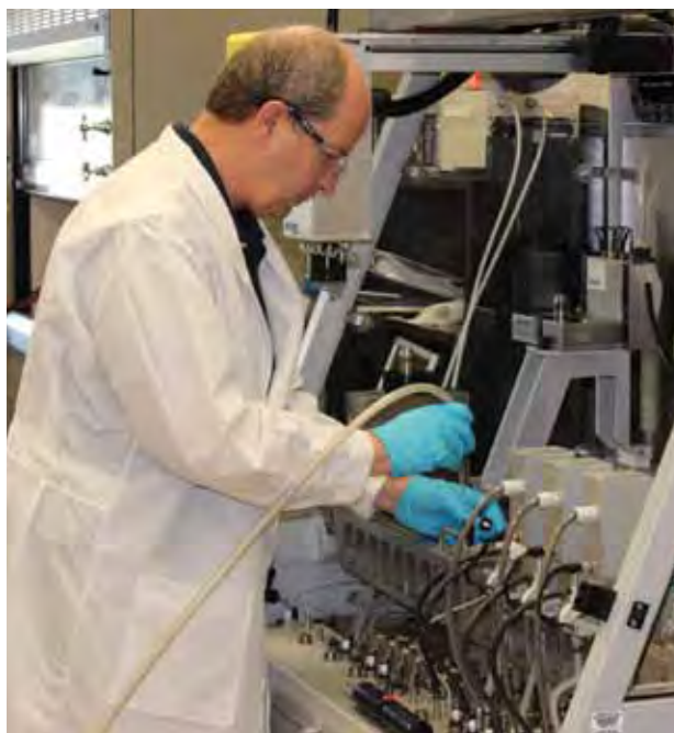
RCCC lab technician, Barry Cunningham, prepares the Chemspeed SLT100 for the high-speed polymer synthesis of polycarbonates at the New Jersey Center for Biomaterials.
