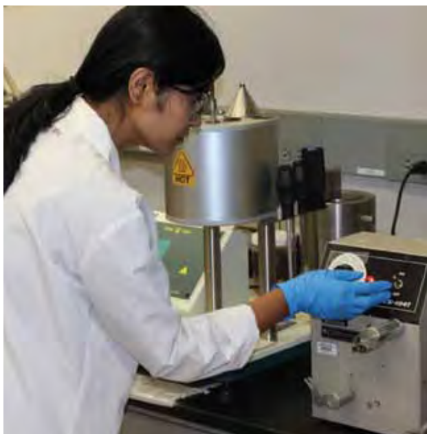
RCCC Postdoc Dr. Divya Bhatnagar operates the extruder instrument in the laboratory to prepare filaments that can be used in braided nerve regeneration conduits.
