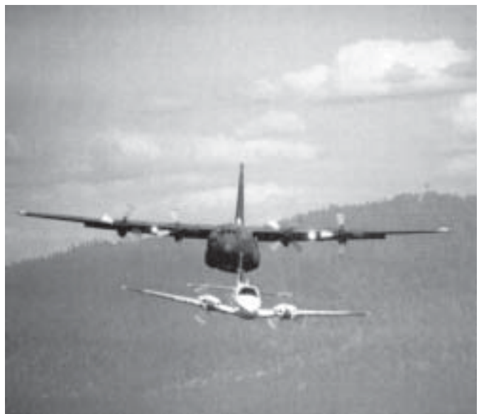
A Beechcraft 58P Baron aircraft that the FS currently uses as a lead plane, guiding an air tanker. FS photo.
