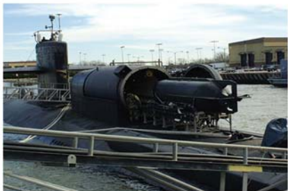
MK VIII MOD SEAL Delivery Vehicle and Dry Deck Shelter
