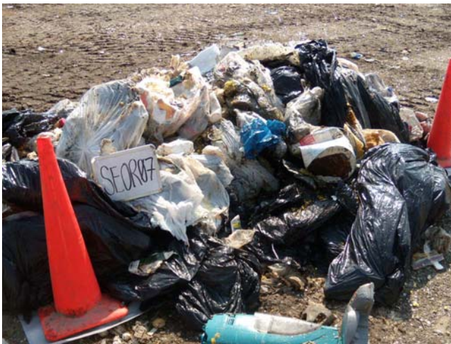
Figure 2-3 Example of a Grab Sample Staged for Manual Sorting
