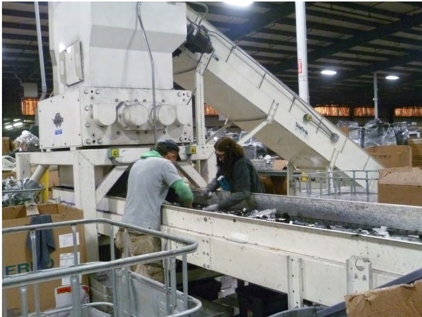
Figure 4. Sorters removing undesirable materials, such as batteries and ink cartridges, at the shredding machine. Photo by NIOSH.
