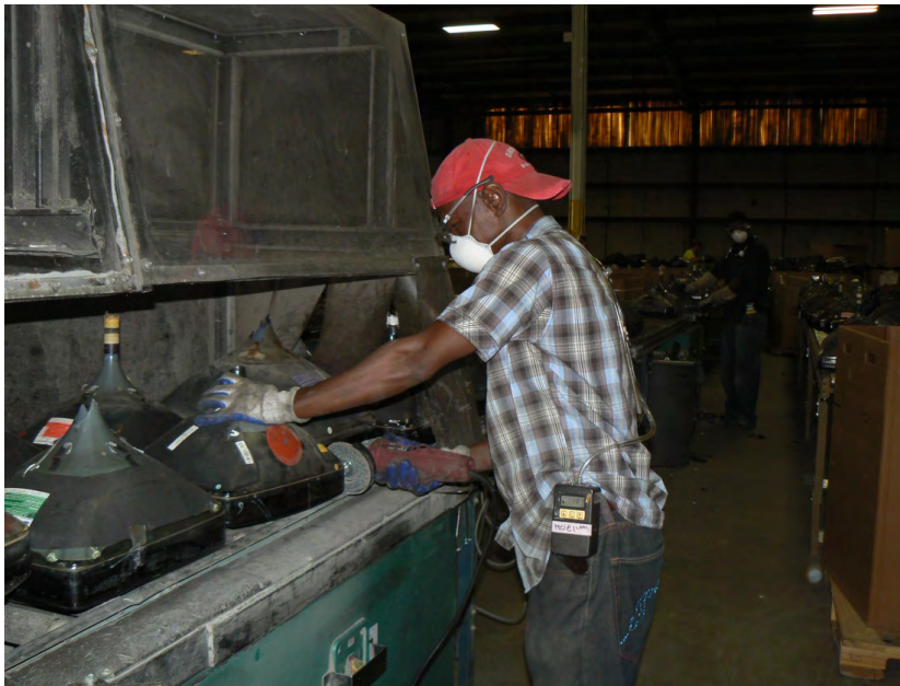
Figure 1. Operator buffing the sides of a CRT on a downdraft table. The strap of the respirator should be under the hat. Photo by NIOSH.
