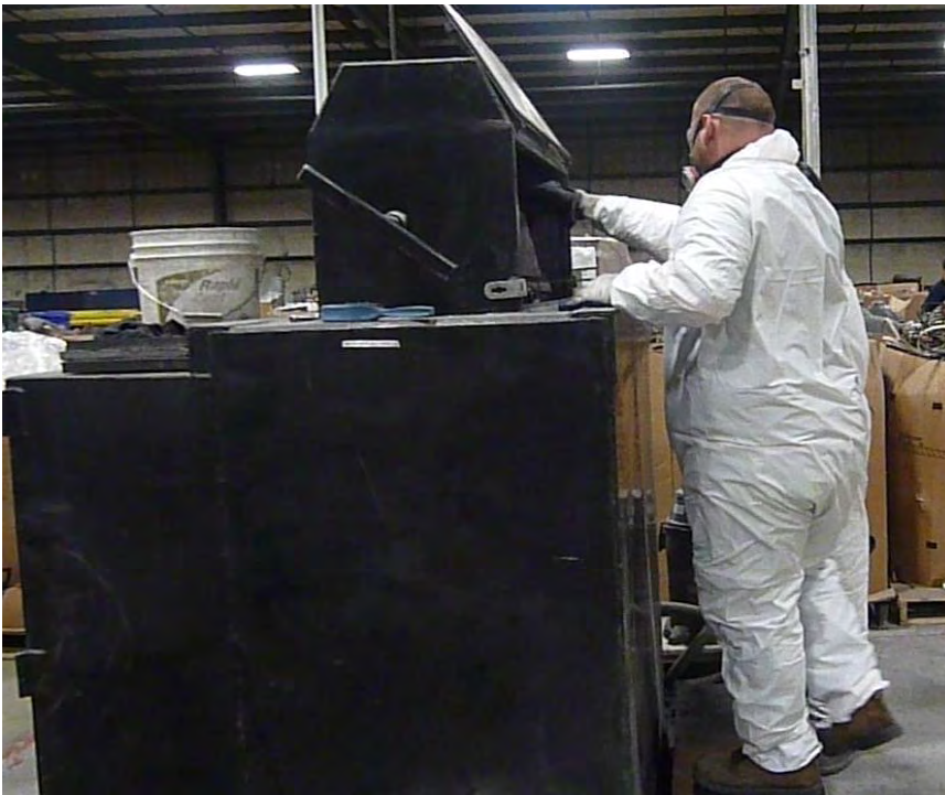
Figure 3. Employee emptying a metal box with broken glass into the mixed glass station. Photo by NIOSH.
