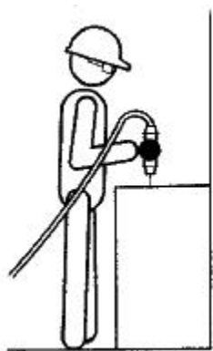
Figure 5. Drawing of an employee using an inline tool in a perpendicular position. Source: http://www.ccohs.ca/oshanswers/safety_haz/power_tools/ergo.html . Date accessed: July, 2014.
