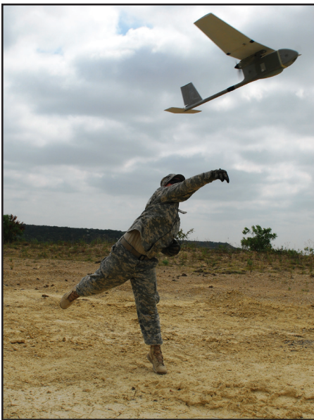
U.S. Army Spc. Ryan Dickinson launches the Raven UAS. (U.S. Army photo by Sgt. Garrett Hernandez/Released)
