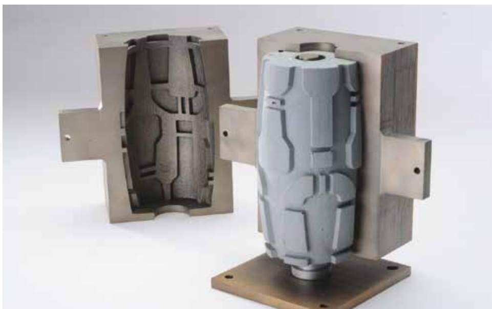
A sample 3D printed sand mold and the resulting cast part from America Makes project led by the Youngstown Business Incubator.
