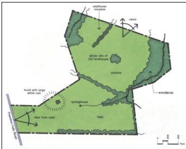
Figure A-1 Sample Constraints and Opportunities Plan showing significant viewsheds, natural and cultural features
