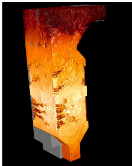
Boiler Simulation Facility temperature field demonstrating the gas temperature field from a typical large eddy simulation.
