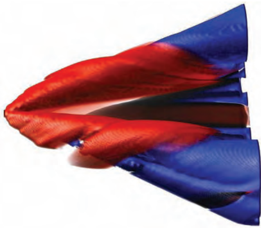
Figure 1. Visualization offers the ability to “see the unseeable.” This image shows visualization of coherent flow structures in a large scale delta wing dataset: Volume rendering of regions of high forward (red) and backward (blue) Finite Time Lyapunov Exponent. Coherent structures appear as surfaces corresponding to the major vortices developing over the wing along the leading edge. 4 Occlusion is a limitation that can be addressed with cropping or clipping. (Image courtesy of X. Tricoche, University of Utah and C. Garth, University of California – Davis)
