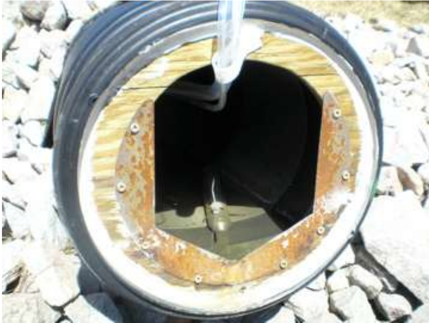
Figure 4-14. Inflow pipe to bioretention area equipped with compound weir and bubbler for flow measurement. Water quality sampling tube and strainer are visible inside pipe.
