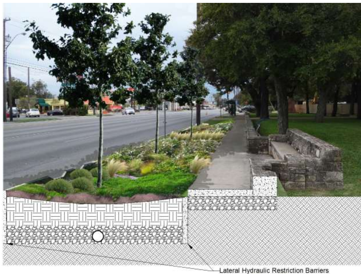
Figure B-11-19. Lateral hydraulic restriction layers in a roadside bioretention area prevent horizontal seepage while allowing infiltration at a safe depth.
