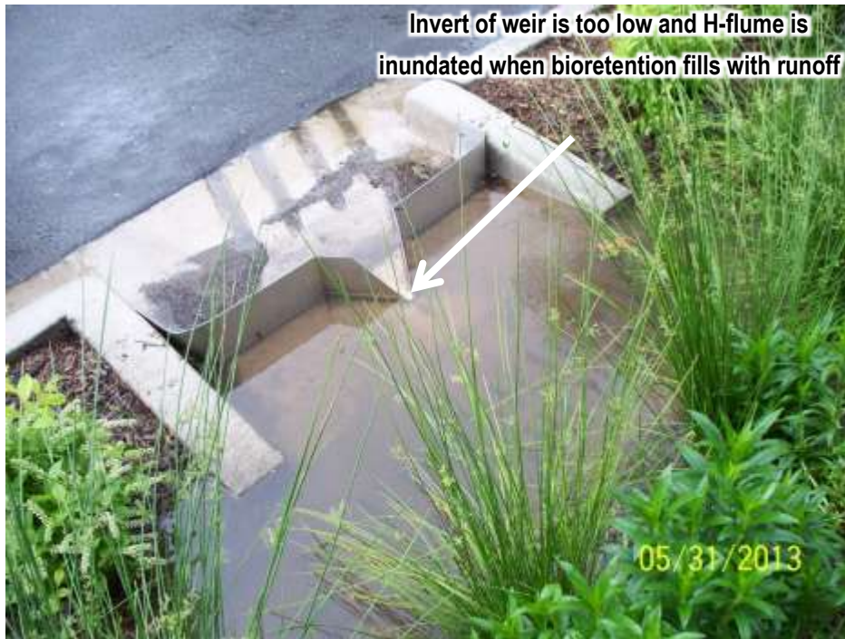
Figure 4-19. Poorly installed H-flume at the inlet to a bioretention area in which the invert of the weir is too low and tailwater from the bioretention will interfere with measurement.
