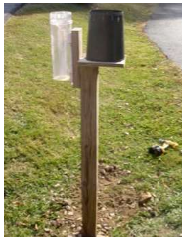
Figure 4-21. Example of manual (left) and tipping bucket (right) rain gauges.
