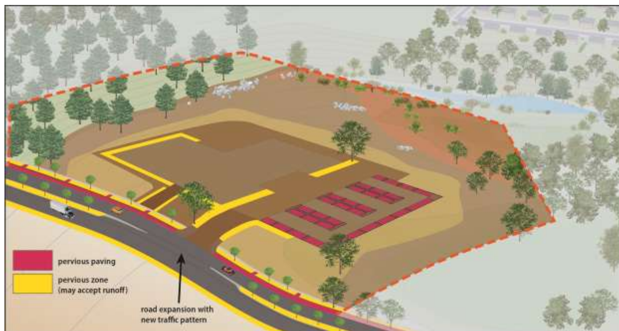
Figure 1-14. Site example demonstrating placement of pervious material (red) and opportunities to minimize connected impervious area (yellow).
