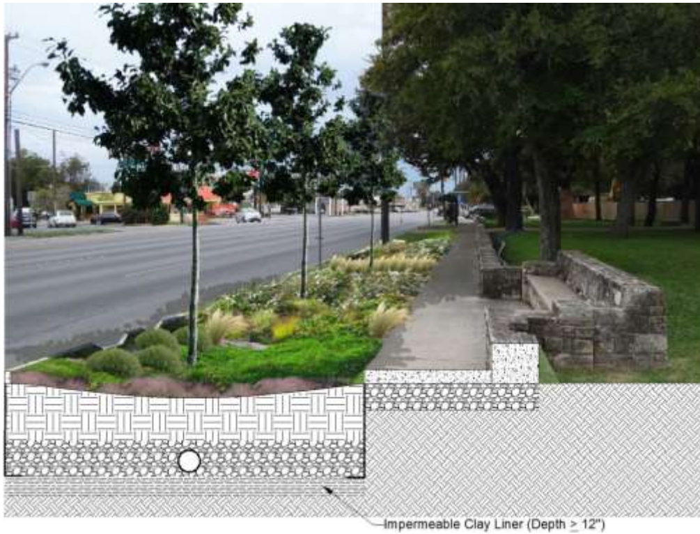
Figure B-11-20. Bioretention area with clay liner and lateral hydraulic restriction barriers.
