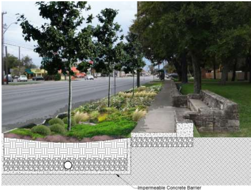
Figure B-11-22. Bioretention area completely lined with concrete barrier (planter box).
