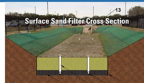
A surface sand filter captures and filters runoff diverted from a parking lot at the University of Texas at San Antonio.
