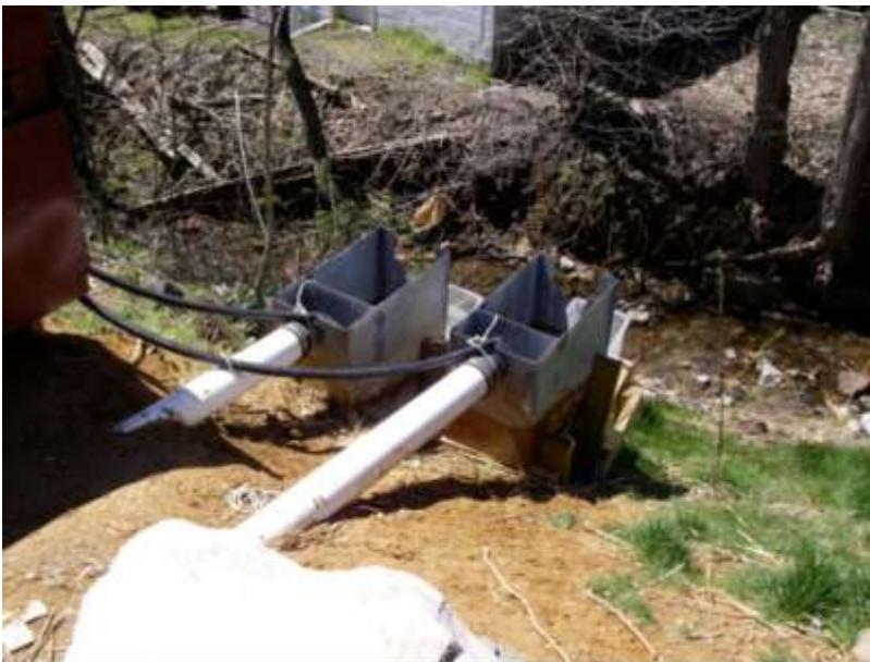
Figure 4-17. Underdrains from permeable pavement equipped with 30° V-notch weir boxes and samplers for flow and water quality monitoring.
