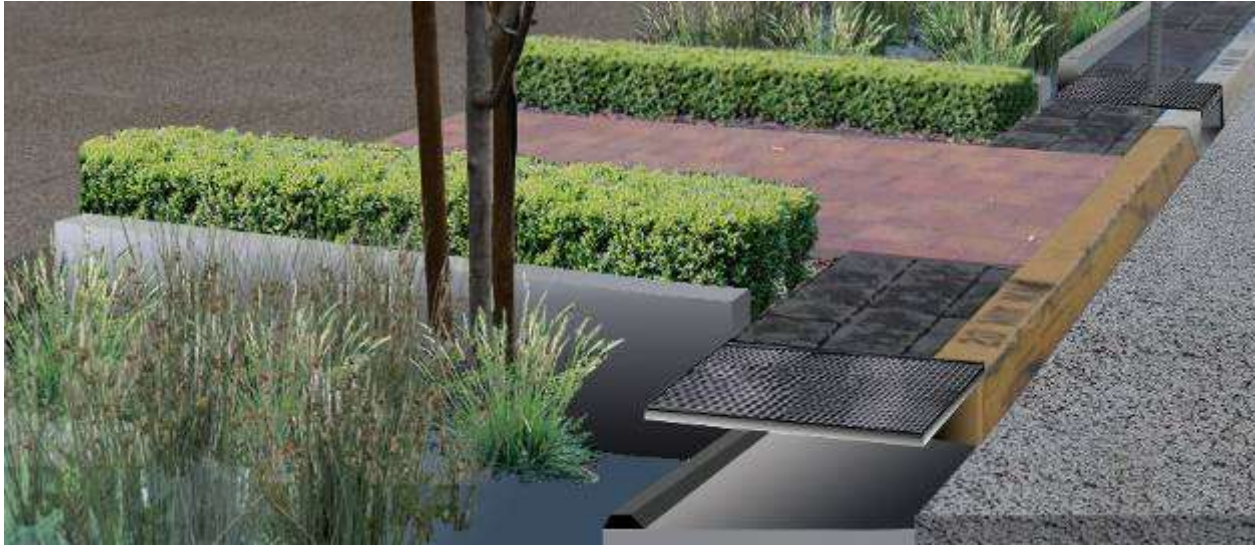
Figure B-11-6. Covered curb cut with a sump.
