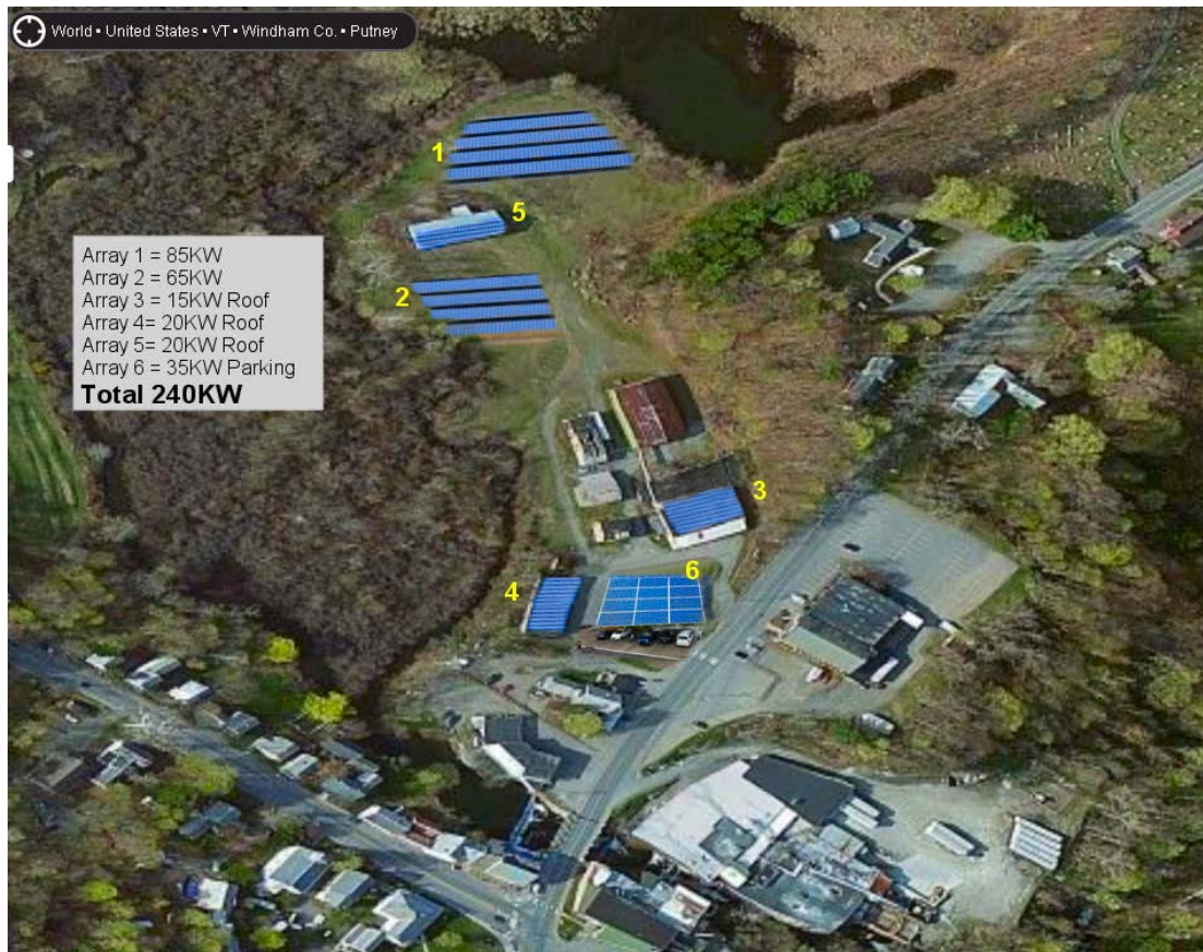
Figure F-1. Potential PV system layouts
