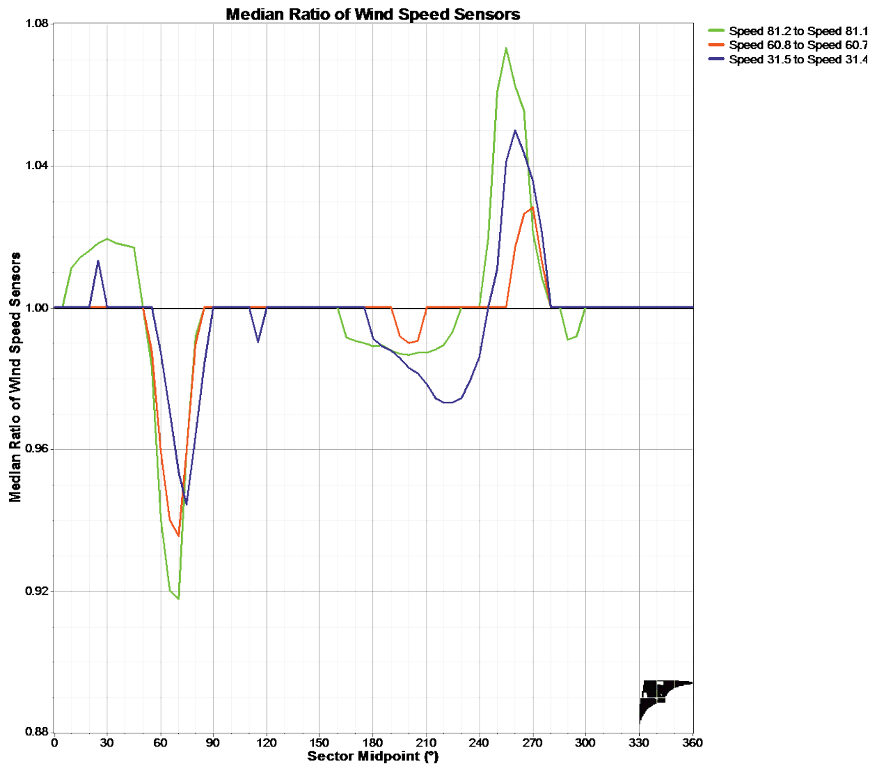
Figure 11. Tower interference on anemometry
