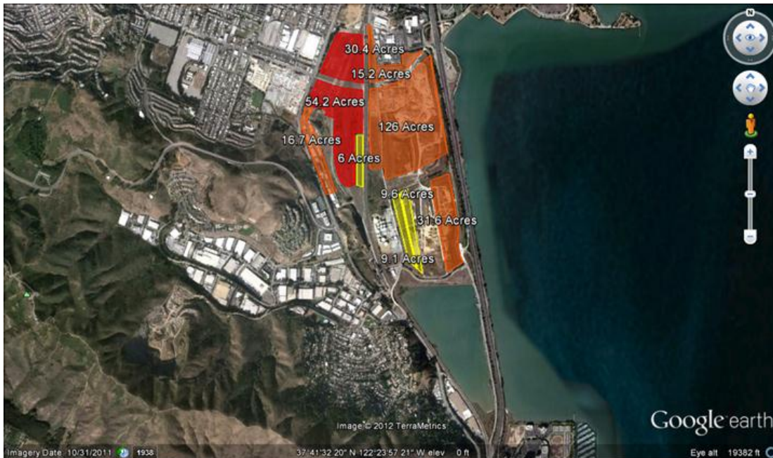
Figure 6. Aerial view of the Developer Option, showing proposed areas for PV at the Brisbane Baylands site (ground-mounted PV in yellow; commercial/retail/light industrial rooftop PV in orange; residential rooftop PV in red)
