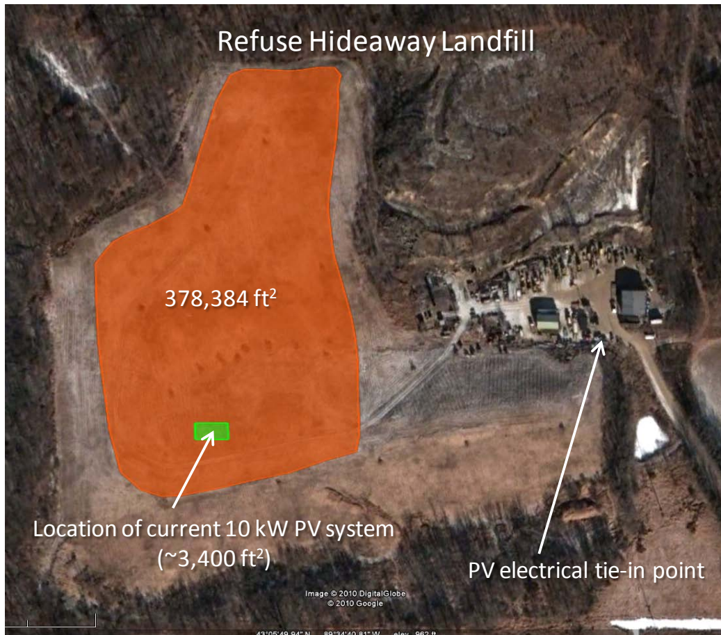
Figure 8. Aerial view of the feasible area (orange) for PV at the Refuse Hideaway Landfill
