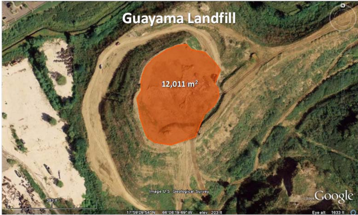
Figure 10. Aerial view of the feasible area for PV at the Guayama Landfill
