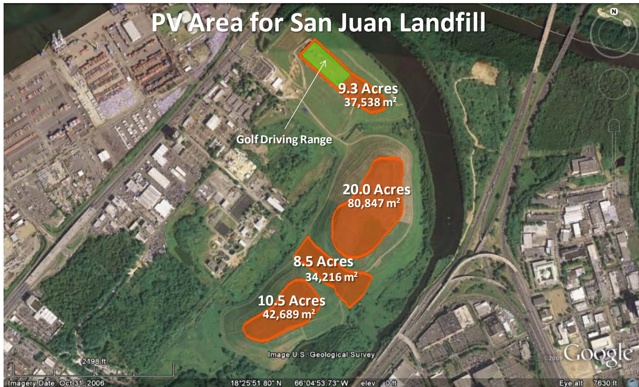
Figure 19. Aerial view of the feasible area for PV at the San Juan Landfill
