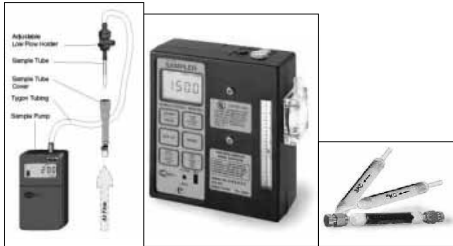
Figure 8. Pumped Sample Collection Method With Adsorbent Media Tubes
