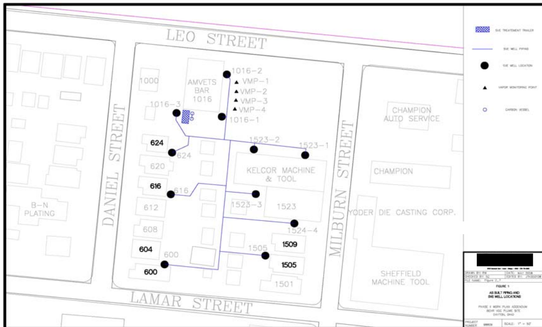
Figure 9 - SVE System Installed at Behr Dayton VOC Removal Site
