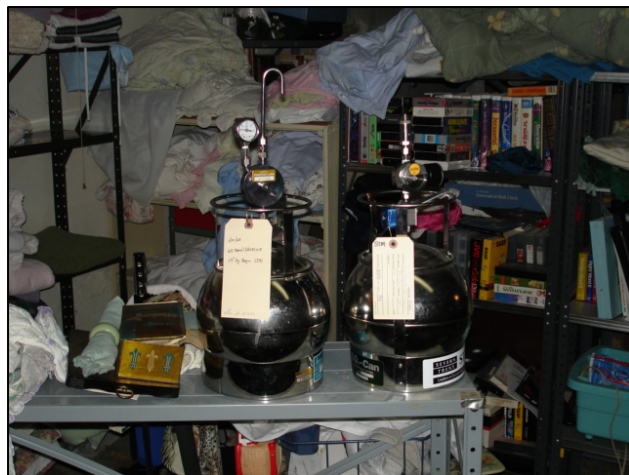
Co-located (Side-by-Side) IA sample collection (left) and co-located SS air sample collection (right)
