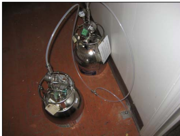
Co-located (Side-by-Side) IA sample collection (left) and co-located SS air sample collection (right)
