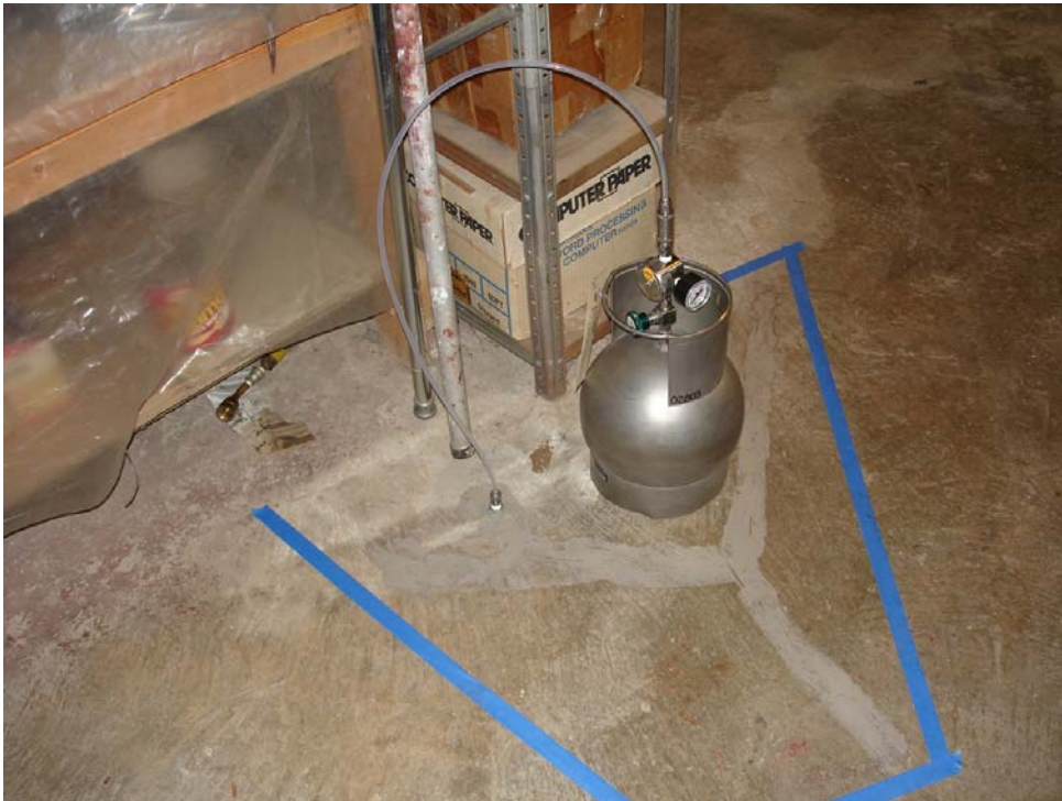
Step 1- Sub-Slab Sampling
