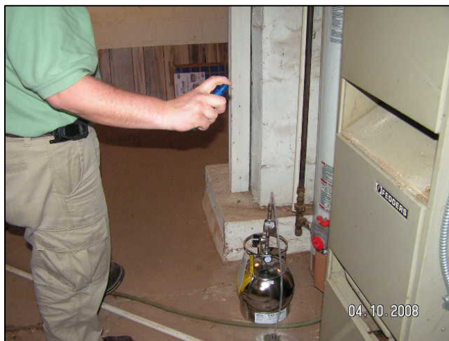
Spraying of isopropyl alcohol as a leak check
