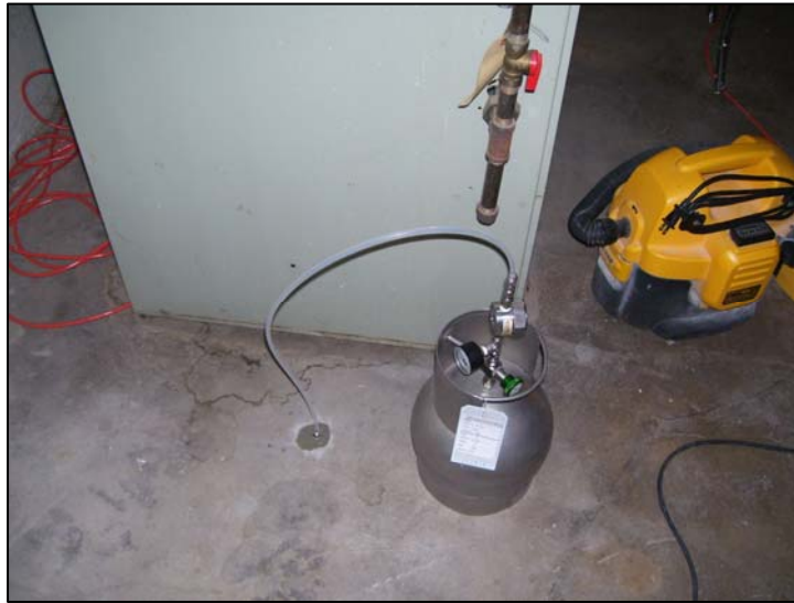
Third Step - Residential SS sampling using sampling probe and SUMMA canister
