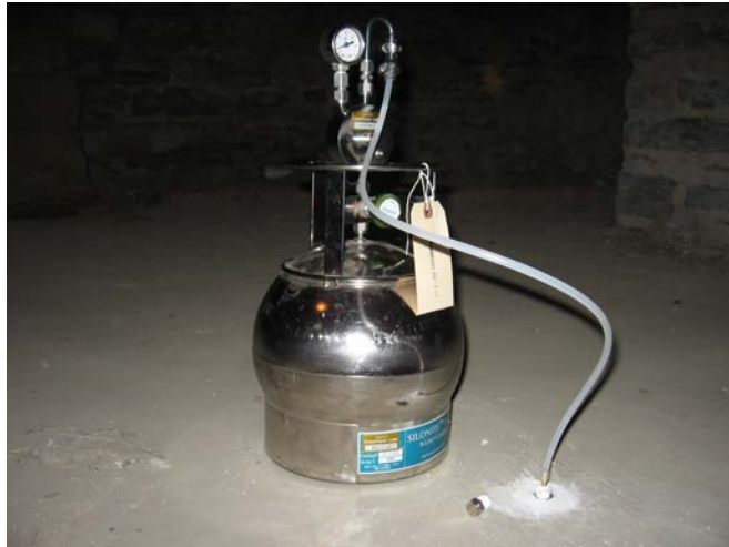
SUMMA canister connected to port and ready for sampling
