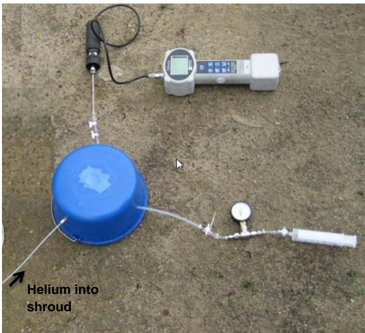
Figure F3. Gas shroud method. Shroud (blue) covering the vapour probe surface seal with line in from helium cylinder, field helium detector, and syringe with vacuum gauge for purging the probe tubing exiting from the shroud.
