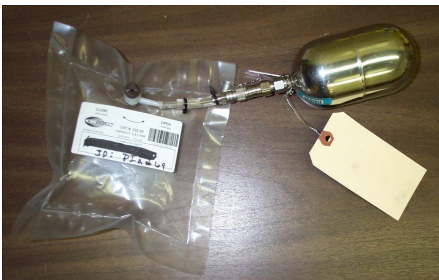
Figure F10 Transferring soil vapour sample from a gas-tight bag into a 400mL canister
