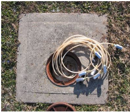
Figure D3 Nested soil gas sample points in a single well: a) Permanent probes with locking cap for repeated sampling; b) Temporary probes which will be removed after sampling
