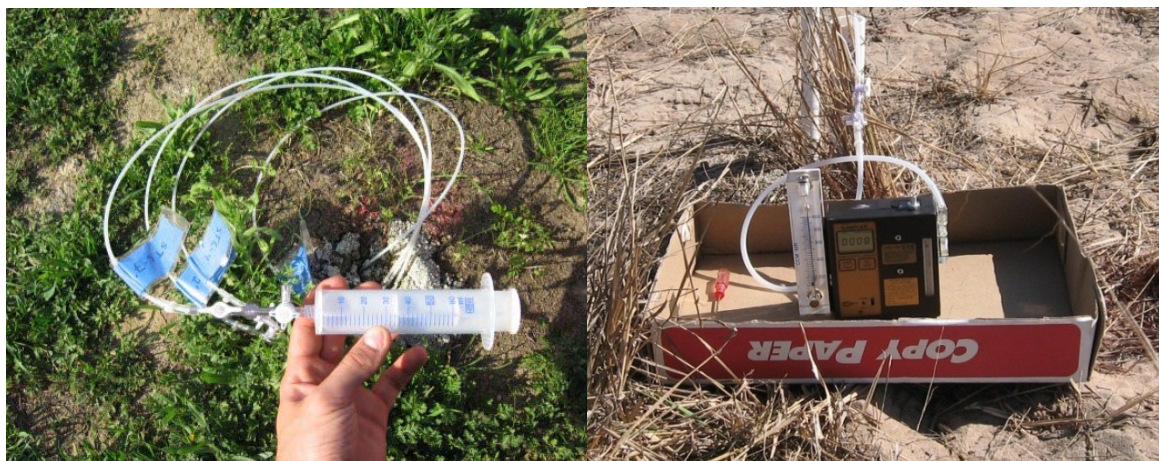
Figure F5. Left: purging with a plastic syringe. Right: purging with a low-flow pump
