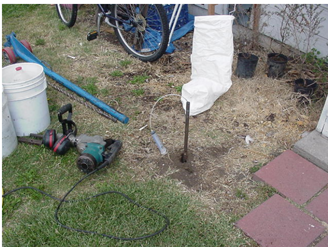
Figure D1 Probe-rod method. Sampling through a steel rod while the rod is in the ground such as with hand probes or direct push systems. Note inert tubing running down the centre of the rod
