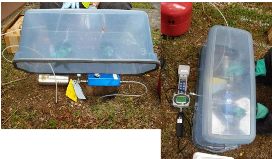
Figure F4. Covering the entire sampling system & probe with a shroud
