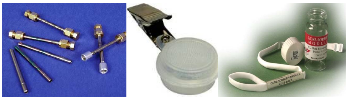
Figure G3 Examples of passive collectors
