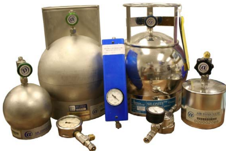
Figure G1 Examples of evacuated passivated canisters and flow controllers.
