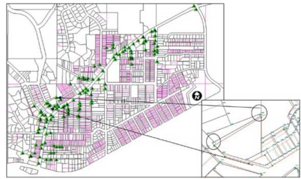
Figure 6. Control points loaded into the fabric for the study area and associated with the appropriate parcel corners
