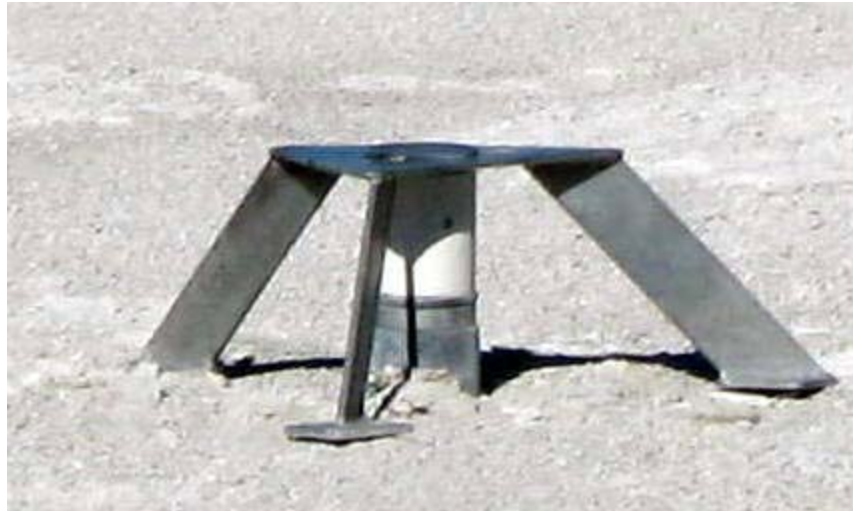
Figure 5. A Height Adjustment Tool is used to measure the height of Sensits and CSCs and to adjust the sensor and inlet height to 15 cm above the soil surface.
