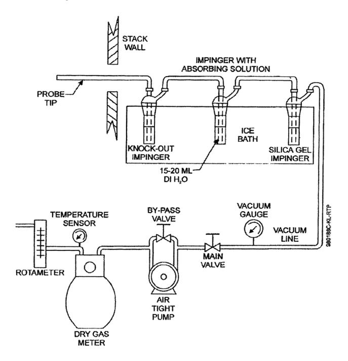
Figure 323-1. Chilled Impinger Train Sampling System
