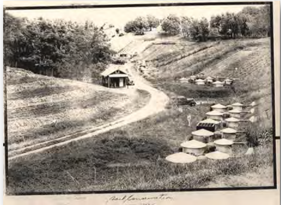
Plots to measure soil erosion at Soil Erosion Station, Mayagüez, PR. (Finca Las Ochenta, adjacent to PR Zoological Park)
