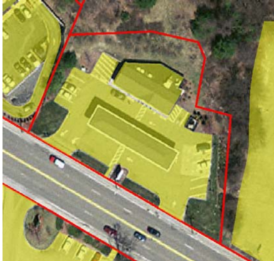
Figure 6.2: Example of Non-Residential Parcel Impervious Area
