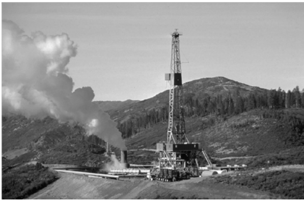
Figure 2: Rig at The Geysers geothermal field in in Middletown, California. This EGS demonstration project, funded by DOE and cost-shared with industry, has shown the potential to produce 5 megawatts from an engineered reservoir in a deep, impermeable, and unproductive rock body, with far greater additional potential at this site. (Photo credit: Calpine; Geothermal Technologies Program 2012 Peer Review)
