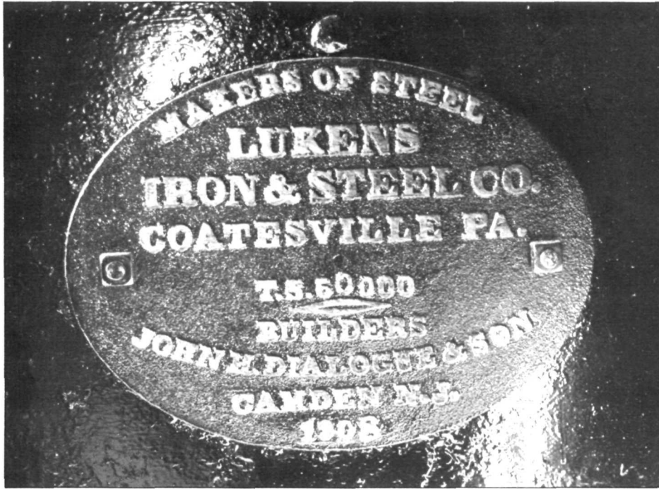
FIGURE 13: Builder's plate in the engine room of the 1908 steam screw tugboat Hercules . (Photo credit: Stephen A. Haller, NPS)
