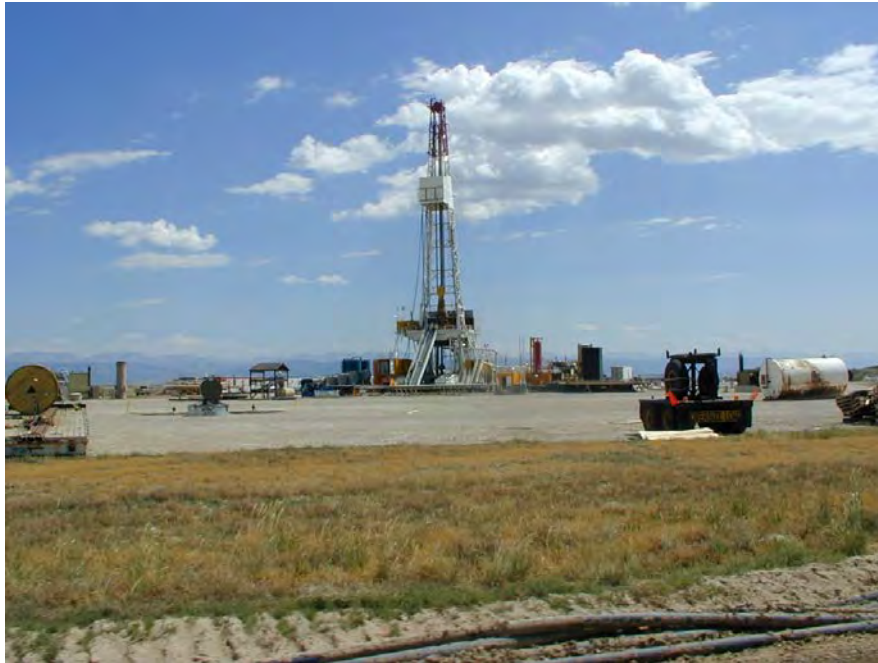
Figure 1. A 3.8 acre gas exploration well pad near Pinedale, Wyoming. The un-vegetated area around the drill rig will be reclaimed after exploration is completed.
