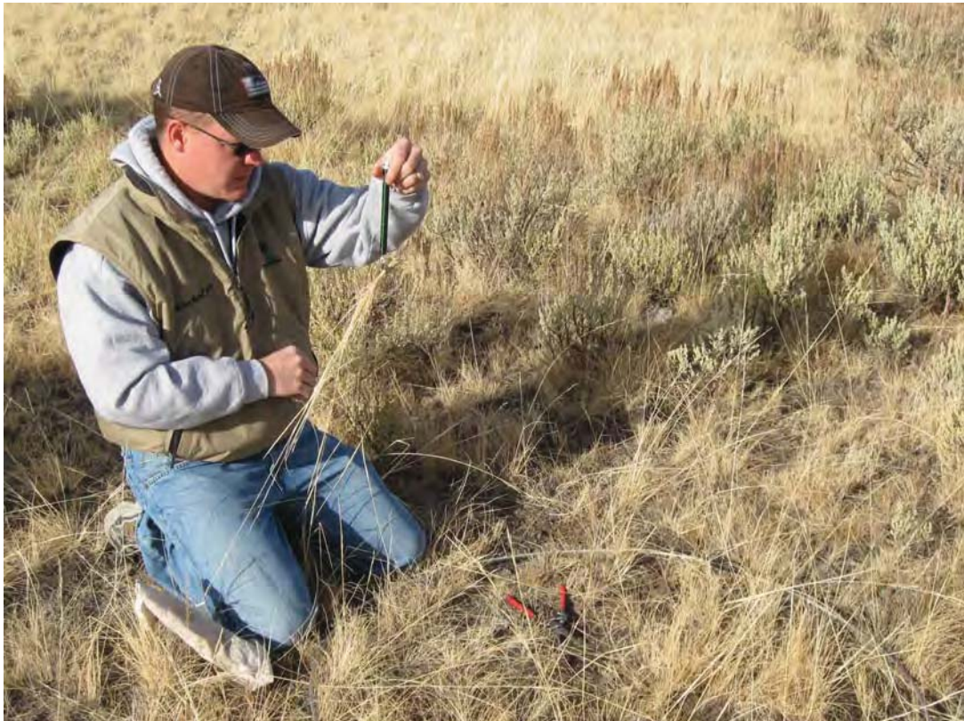
Collecting Production Data Using 9.6 ft 2 Hoop, Clippers, Scale, and Cloth Bag; Photo: Brendan Brazee, NRCS, Boise, ID
