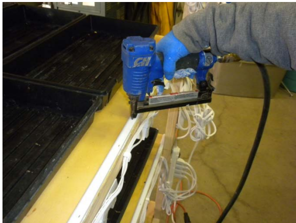
Figure 9. Installing shoe molding on side of shelf
