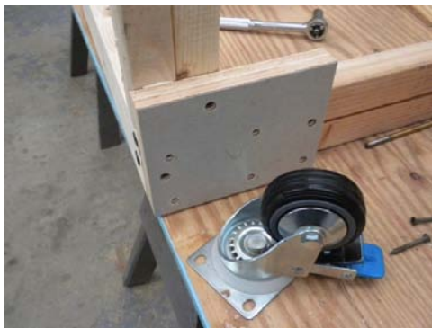
Figure 6. Countersink holes in castor support
