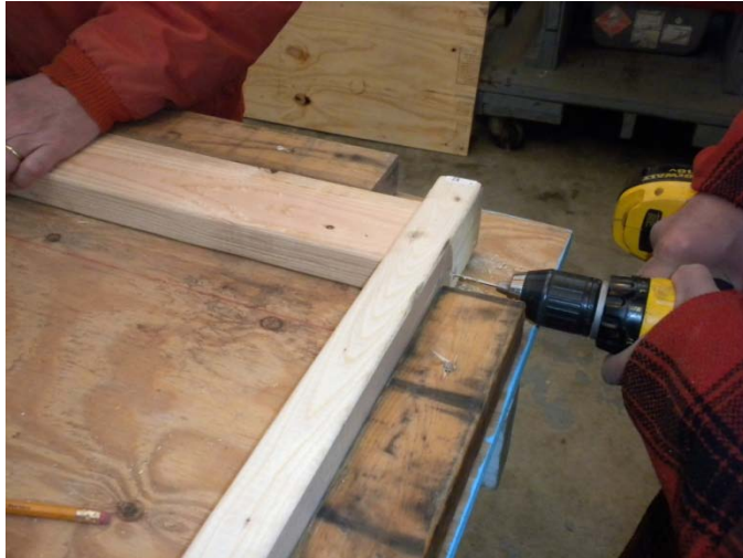
Figure 3. Using jig to assure square and level corners for shelf support
