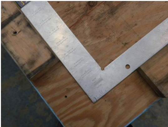
Figure 1. Creating a jig to assure square corners
